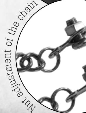
Fasten the chain to the holes in the side of the Grill-Smoking Oven between the upper and the lower part. Adjust the nut in the chain so that the chain can move freely, and fasten the chain from the inside of the Grill-Smoking Oven with a flange nut in the upper and lower part. Tighten the screws with the spanner.
